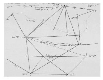
Fig.7: The triangulation sketch of F. L. Pfyffer, found in one of his letters to Micheli Du Crest. The long dotted zigzag line in the upper part was measured using metal chains. Out of these direct measurements Pfyffer determined the length of the baseline MN to 2832 French toises (around 5.5 km).
